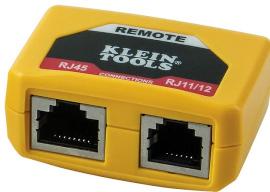
This replacement remote works with Klein's LAN Explorer tester (VDV526-100). Tests RJ11, RJ12 and RJ45 terminated voice and data cables for Miswires, Open-Faults and Short -Faults. The remote stores securely in the tester body.
