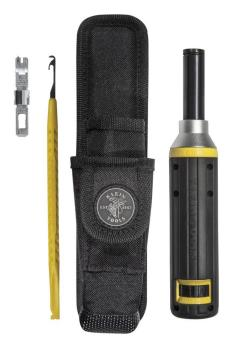
The Cushion-Grip Impact Tool Kit provides everything required to install and maintain 110 and 66 panels, cross-connect systems and wall jacks with secure terminations. Utilizing an optimized two-step impact process, the punchdown tool precisely inserts and then trims off excess wire. The 4-Piece kit comes with punchdown tool, wire pick, blade and pouch.
