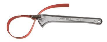
The Klein Tools 18-Inch Grip-It Strap Wrench is completely adjustable for tight-quarters tasks on polished, PVC and glass pipes, fittings, filters, conduit and shafts. The strap is urethane-coated to resist scratching or damaging surfaces and is attached to a lightweight I-beam handle. Also available in 6-Inch and 12-Inch lengths (Cat. No. S6H and S12H).
