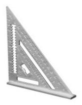
As a saw guide, stair layout tool or rafter tool, Johnson's rafter square will help you get the job done accurately and easily. Its solid aluminum body construction with CNC machined edges provides greater accuracy along with durable chipresistant coating. Use the scribe notches for marking and ripping lumber, and handy markers that measure 2x4 board dimensions of 1-1/2", 3" and 3-1/2". This square also has deep cast-in graduations that will never peel off, wear off, fade or smudge.
