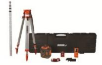
The 99-027K is great for large jobsites with its 2000' working diameter. If you're working large jobs and don't need a rotary with slope, this model is perfect for you. With accuracy of 3/16" per 100', this rotary is suitable for any layout work you'll encounter. And its IP66 construction makes it suitable for even the dustiest jobsites you'll encounter. It also features a hard-shell contractor's carrying case to hold all system components.
