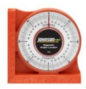
Simplify angle measurements with Johnson's magnetic angle locator. Featuring a high-impact molded body and an extrastrong ceramic magnet, it effortlessly adheres to ferrous metal surfaces. The V-groove edge ensures a perfect fit on pipes and conduits, while easy-to-read increments display 0-90° in all four quadrants on a durable acrylic lens. For added convenience, one side has inch graduations and the other has metric graduations.
