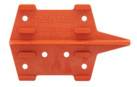
Johnson's deck board spacing tool is an easy to use, one-piece tool for the most common deck board sizes. It evenly spaces dry or green deck lumber - allowing enough room for expansion and contraction and eliminating guesswork. The spacing tool features a durable, high-impact body and 1/8" and 3/16" spacer edges, while the included layout guide provide easy guidance for 2x4 and 2x6 decking.
