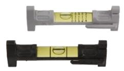
Two is better than one! These 3" line levels' lightweight design reduces line sag, for an accurate reading every time. They are also highly durable thanks to their impact-resistant Structo-Cast® construction and feature unrestricted hooks that allow for easy movement. The impact-resistant Multi-Pitch® vial also reads slope in 1/8" per foot increments.
