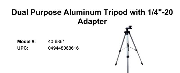
Johnson's dual-purpose aluminum tripod, with an adapter that reduces threads from 5/8" - 11 to 1/4" - 20, attaches quickly and easily to laser or optical levels and extends to a maximum height of 65". It also includes an elevating column with fine adjustment knobs for maximum accuracy, while the adjustable tripod feet make this an ideal choice for outdoor or indoor jobsites. With the included nylon carrying bag with a shoulder strap, this tripod has everything you'll need to get up and running!
