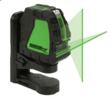
Green beam is 400% more visible than red beam, self-leveling, projects one horizontal, vertical or cross-line beam separately or simultaneously, Visual out of level indicator, Multi-functional elevating magnetic bracket with rare earth magnets for use on walls, metallic surfaces or tripod, While on the bracket, and the laser can be raised or lowered 2-1/2" and rotate 360°.
