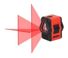
Johnson's 40-6648 Self-Leveling Cross & Line Laser combines the features of a cross-line laser with an additional 90 degree plumb line useful for checking square reference of beams, posts, or any other object. A 1/4"-20 tripod thread and manual mode also let you project orthogonal lines at any angle, for stairs and other non-level applications.
