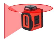
Johnson's 40-6606 Self-Leveling 360° Laser displays a full horizontal line 360 degrees around the tool, plus a plumb layout line that intersects the 360 to help you layout your jobsite quickly and accurately. A 1/4"-20 tripod thread and manual mode also let you project orthogonal lines at any angle, for stairs and other non-level applications.
