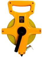
Make your next large measuring job easy with this metric/inch fiberglass long tape. The 30m/100' long tape features a 1/2" blade with both metric and inch graduations. And it was built to last, with a high impact ABS case and a durable PVC-coated blade that resists abrasion. The tough blade hook keeps the blade from slipping during use, ensuring your measurements are accurate.
