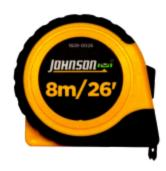
Measure with confidence with Johnson's 8m/26' measuring tape. The sturdy 1" blade features metric/inch graduations on the top side and metric graduations on the bottom side, while the blade hook's triple rivets keeps the blade from slipping during use. For durability, the nylon-coated blade resists abrasion and the rubberized co-molded case absorbs shock and provides a non-slip grip.
