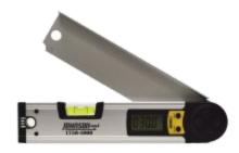
Check and transfer angle measurements easily and accurately with Johnson's 10" digital angle locator. This tool easily measures and clearly displays angles and will make your job go faster, saving you time and money. The digital display shows your angle measurements in degrees from 0° to 225° and gives you the option of taking measurements of absolute or relative angles with the simple press of a button.
