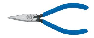
These lightweight, Electronics Pliers feature a long, slim nose for delicate, precision assembly work. The jaws are knurled for sure wrapping and looping of wire. Spring-loaded for self-opening action with curved handles for greater tool control. Made in the USA of forged steel for long life.
