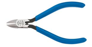
With Klein Tools' 4-Inch Electronics Pliers, you can easily work in confined spaces. The short jaws and beveled cutting edges permit close cutting of wire. These diagonal cutting pliers feature a hot-riveted joint that ensures smooth action and no handle wobble.
