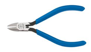
These Electronics Pliers have a tapered nose for easy working in confined areas and close tip cutting. The short jaws have beveled edges for semi-flush cutting of wire. The induction hardened cutting knives and hot-riveted joint ensure smooth action and long life.
