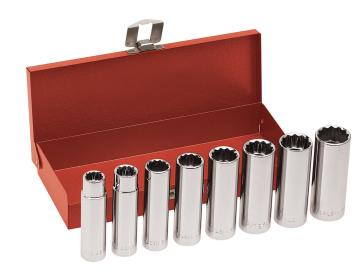
8-Piece 1/2-Inch Drive, Deep-Socket Wrench Set. Comes with a red hinged metal box. The set has eight 12-point deep sockets: 1/2-Inch, 9/16-Inch, 5/8-Inch, 11/16-Inch, 3/4-Inch, 13/16-Inch, 7/8-Inch, and 15/16-Inch.
