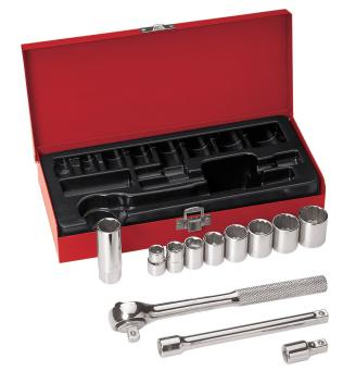
This 12-piece Wrench Set includes four 6-point and four 12-point sockets. 6-point socket sizes include 3/8-Inch, 7/16-Inch, 1/2-Inch and 9/16-Inch. The four 12-point sockets span 5/8-Inch, 11/16-Inch, 3/4-Inch and 13/16-Inch sizes. Also, includes a 5/8-Inch spark plug socket, two extensions and a ratchet. Keep all of pieces together in a compact hinged metal box.
