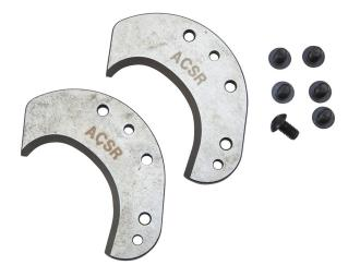
These Klein Tools replacement blades fro the ACSR ratcheting cable cutter come with two blades and six screws. They are easily replaced by simply removing 3 screws per blade. The blades are equipped to cut up to 477 MCM ACSR multi-strand.
