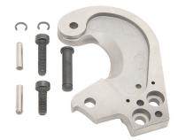
This replacement blade set for the Ratcheting ACSR Cable Cutter (63607) cut copper, aluminum and ACSR. Forged, heat-treated, shear-type cutting blades are made of hardened steel for sharpness and long life.
