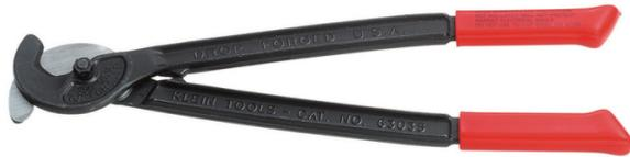
This Utility Cable Cutter features shear-cutting blades that cut 350 MCM Copper and 350 MCM Aluminum cable. Made from forged steel with black-oxide finish for long life. Shear-type hook jaws grab and hold cable. Non-slip vinyl grips on 16-Inch handles keep this tool safely in your hands. Does not cut steel or ACSR.
