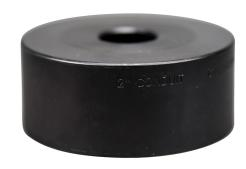
Easily punch holes for 2-Inch EMT conduit. Has a maximum capacity of 10 gauge mild steel. Cuts aluminum, fiberglass and plastic as well.
