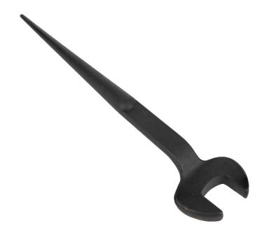
Forged from select alloy steel, the Klein Tools 1-1/2-Inch Nominal Opening Spud Wrench is designed to withstand high-leverage and heavy loads. It's designed for use with 1-Inch bolts and U.S. regular nut types. The extra-duty head area gives maximum strength and durability. Plus, the continuous taper of the handle makes it easy to line up bolt holes.
