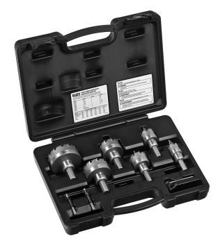
This hole cutter kit cuts quick, precise holes in a variety of materials. Includes six commonly used size plus two extra pilot bits. Integrated flange prevents the operator from drilling beyond the sheet metal. Split point pilot drill bit prevents bit walking.
