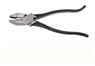
Klein Tools Ironworker's Pliers have aggressive teeth for a strong grip when twisting, snipping and pulling soft annealed rebar tire wire. The knurled jaws aid in easy twisting and turning. These pliers feature a hook-bend in the handle for added grip and leverage. Unique handle tempering helps absorb the "snap" when cutting wire.
