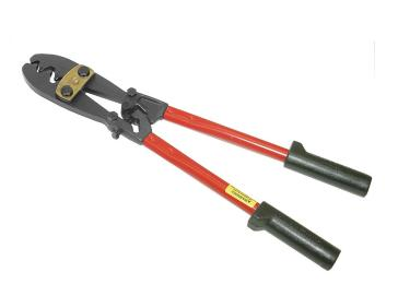
Use this crimping tool to crimp 6 - 4/0 AWG lugs and terminals. High-leverage handles and compound-action mechanism offer superior mechanical advantage. Ultra-comfortable hand grips for easy use and minimal fatigue. Adjustment screw allows user to control crimp depth.
