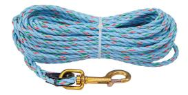
Klein Tools Polypropylene Hand-Line with Snap Hook is made with 5/16-Inch (8 mm) three-strand polypropylene 75-Foot (22.9 m) rope spliced to the eye of a swivel hook. The hook is a forged steel hook with swivel clevis and quick-acting plunger-style latch.
