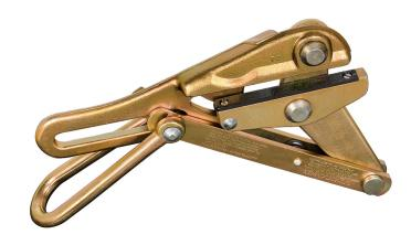
Designed for use on aluminum, copper, weatherproof coated wire, PVC covered conductors and messenger and guy strand. The Chicago style grip was designed for cable sizes from 0.16-Inch to 0.55-Inch (4.06 - 13.97 mm). Double -InchV-Inch grooves give four-point contact, reducing chance of slipping and providing proper alignment of wire and cable.
