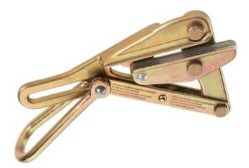
Designed for use on aluminum, copper, weatherproof coated wire, PVC covered conductors and messenger and guy strand. The Chicago style grip was designed for cable sizes from 0.218-Inch to 0.55-Inch (5.5 to 13.9 mm). Double "V" grooves give four-point contact, reducing chance of slipping and providing proper alignment of wire and cable.
