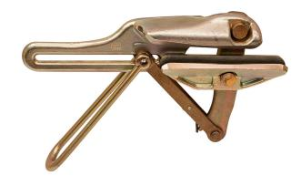
The Klein Tools Chicago® Grip - Dual Conductor Trans is designed specifically for VR2® (vibration-resistant) and TransPowr® T-2® dual conductor twisted pair cables. The machined upper and lower jaws eliminate scoring or damage to second conductor by contouring to second conductor. The round jaws are shaped to provide maximum contact with circumference of cable and prevent cable deformation.
