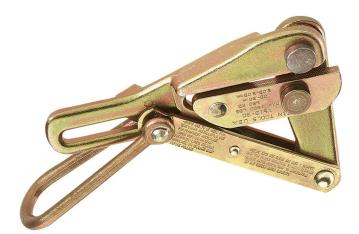
Klein Tools' 1613 Series Bare Wire Chicago Grips are designed to work with solid and stranded bare wire from 0.08-Inch to 0.20-Inch (2 mm to 5.1 mm). All Klein grips are manufactured from custom drop-forged steel that is machined and heat treated for excellent durability. Each grip is individually hand inspected and actuated for proper function. Grips are also rigorously tested and pulled to rated load to ensure the highest quality and reliability.
